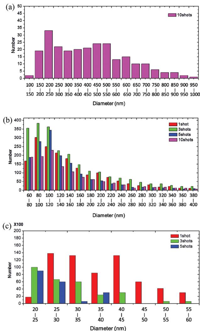
Fig. 3 Particle size distribution within a  $10 \times 10 \mu\text{m}^2$  area of Ag NPs formed on (a) Si, (b) glass, and (c) filter paper.
