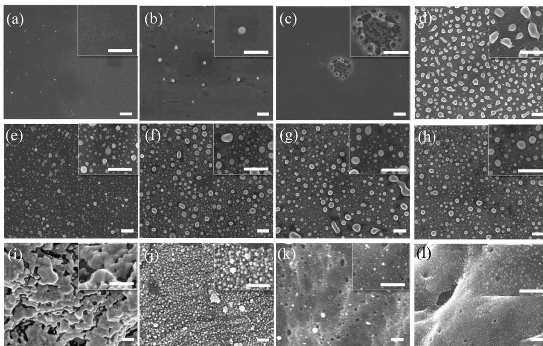
**Fig. 2** SEM images of the distributions of Ag NPs formed on (a–d) Si, (e–h) glass, and (i–l) filter paper after different numbers of shots of KrF laser illumination. For Si and glass, the numbers of shots were (from left to right) 1, 3, 5, and 10; for filter paper, the numbers of shots were (from left to right) 0, 1, 3, and 5. Inset: enlarged images of the NPs. Scale bars: (a–h) 1  $\mu\text{m}$ ; (i–l) 200 nm.
