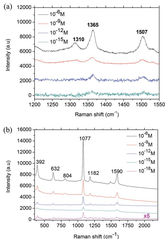
Fig. 7 SERS spectra of various concentrations of (a) R6G and (b) 4-ATP dried on Ag NP-containing SERS filter paper, demonstrating attomolar detection ability.
