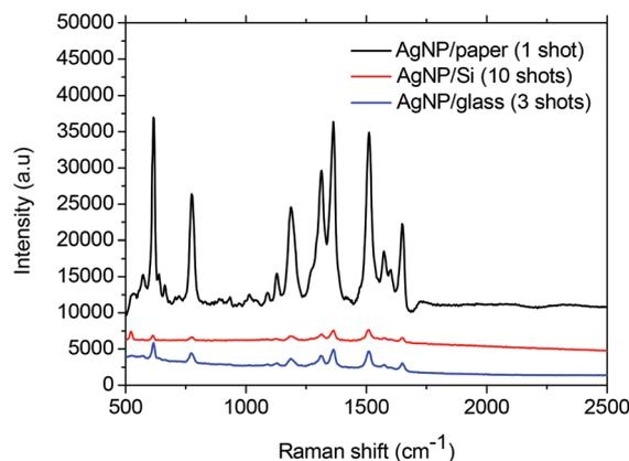
Fig. 4 SERS spectra of  $20 \mu\text{L}$  R6G ( $10^{-6}$  M) droplets that had been dried on various hydrophobic SERS substrates.
